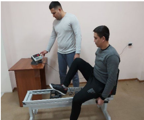
Fig.1. An example of measuring the registration of special speed-strength indicators of the extensor muscles of the knee joint
